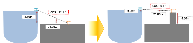
Fig. 15. Effect of raising the height of bitt (case 5)
